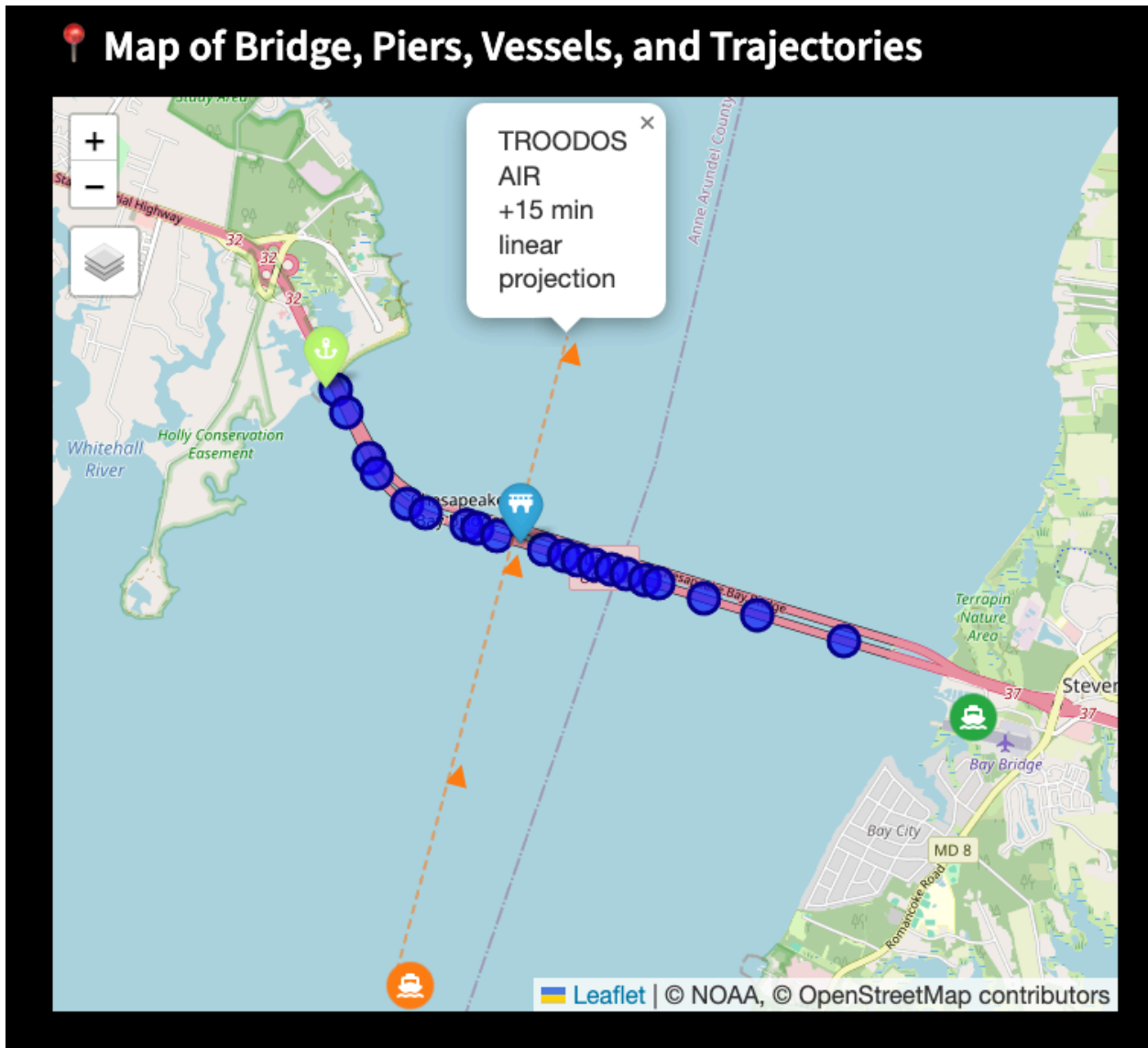
Figure 4 - Click on a triangular arrow emanating from a moving vessel and you will see the vessel's forecasted location at 5, 10, and 15 minutes into the future. The forecast is a linear projection of the vessel's current speed and course.
